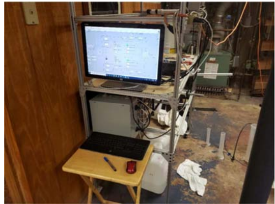
Figure 4. Photograph of Electronics and computer control module.
