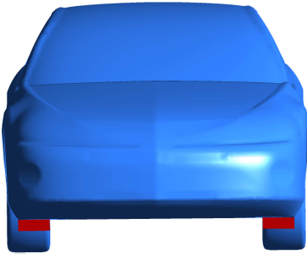
Fig. 2. Full scale vehicle model installed with front wheel spoiler.
