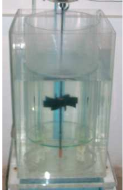
Fig. 1. Stirred tank equipped by a concave blades turbine.
